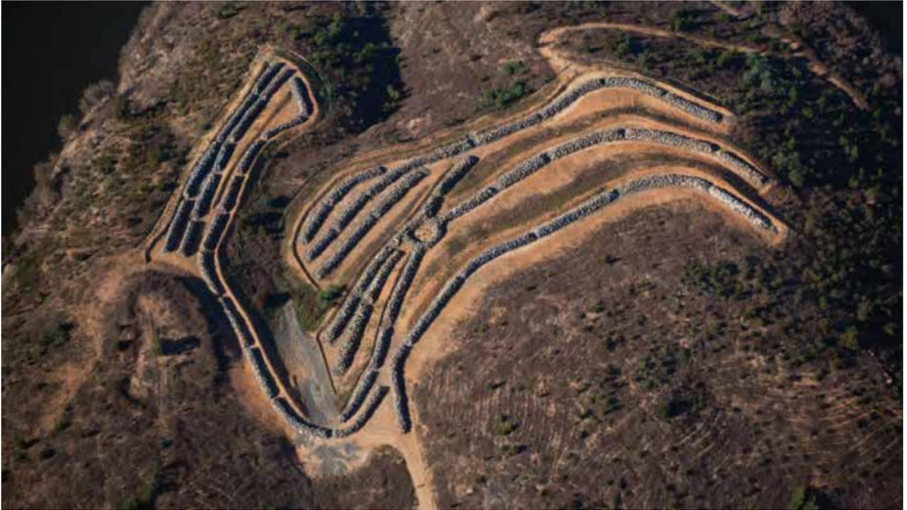
Satellite image of the rock reef artificial habitat constructed within the Enlarged Cotter Dam
