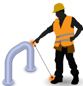
Figure 1. Touch voltage on metallic pipeline
