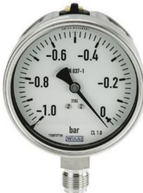
Fig. 13.2 An example of an acceptable analogue vacuum gauge for vacuum testing of sewer mains-to-tie pipe runs at -24 kPa (-0.24 bar)
