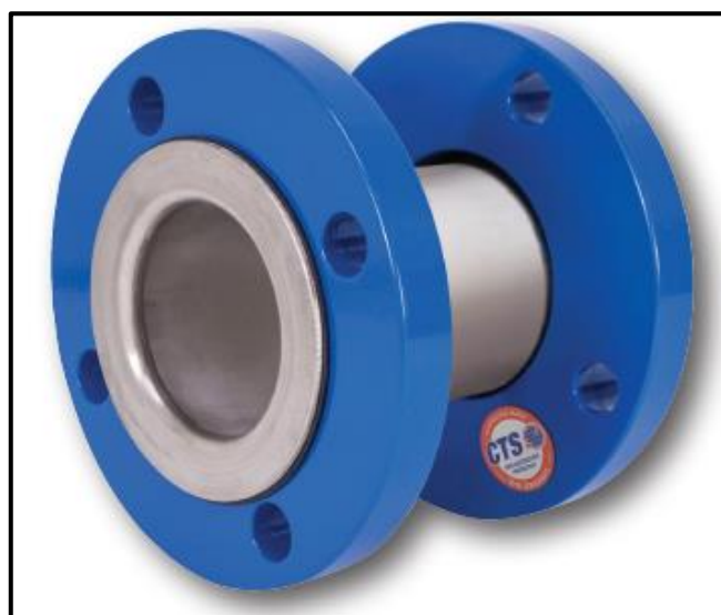
CTS Flanged Pipe Spools – Pre-fabricated (SS316 SCHED 10S pipe and powder coated carbon steel flanges with EPDM insulators)
