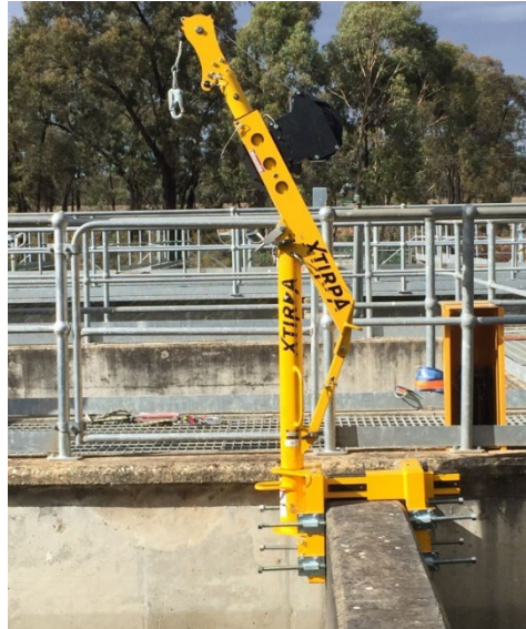
Figure 2.7.5 An example of a davit clamping zone on a parapet wall
