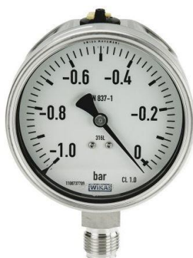
Figure A.1 - Example of an acceptable analogue pressure gauge for a test pressure of -24 kPa (-0.24 bar)
