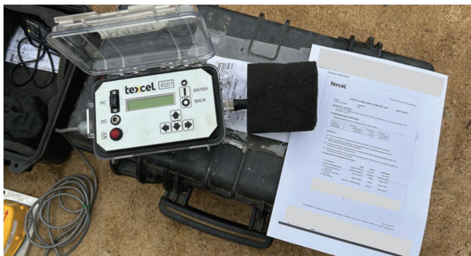
Figure 5.4.1 Example vibration monitoring instrument and certification for calibration
