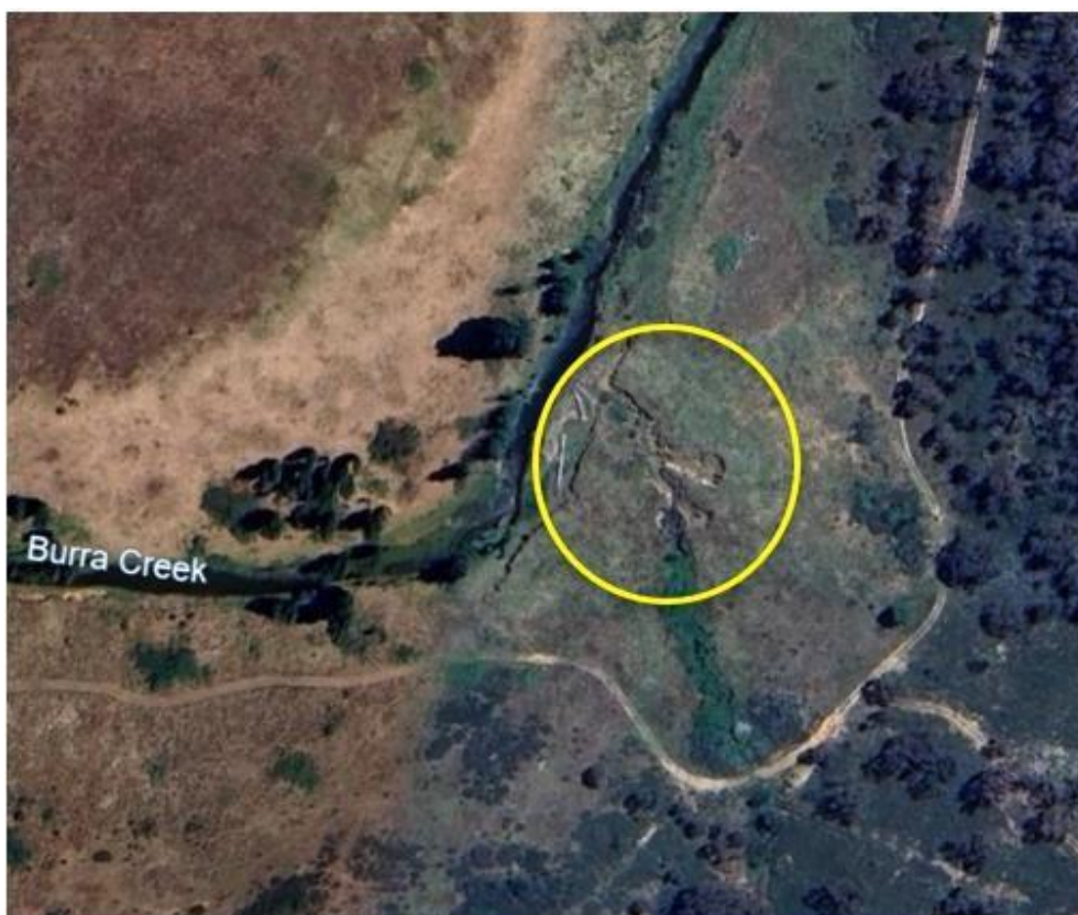
Figure 19. Aerial view of the MZ7 (G9) erosion site on the true right bank of Burra Creek. Image shows active gully incision extending from the roadside toward the creek (parts of the lower gully are obscured by blackberry cover). The site drains directly into Burra Creek, posing a sediment risk to Googong Reservoir.
