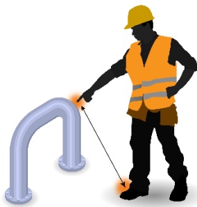
Figure 1.1.1: Touch Voltage on Metallic Pipeline
