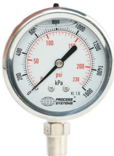
Fig. A.1 Example of an acceptable analogue pressure gauge for hydrostatic testing at 1400 kPa (14 bar)
