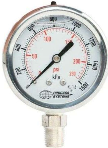
Appendix D 1 An example of an acceptable analogue pressure gauge for hydrostatic testing of water mains-to-meter pipe runs at 1400 kPa (14 bar)
