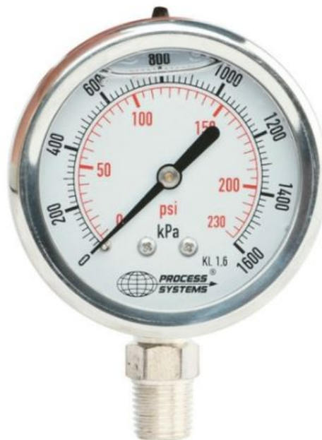
Fig. 6.1 Example of an acceptable analogue pressure gauge for hydrostatic testing at 1400 kPa (14 bar)
